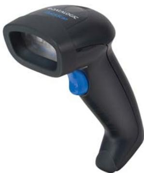
It is possible to connect a USB barcode reader to fill the M400 fields.
